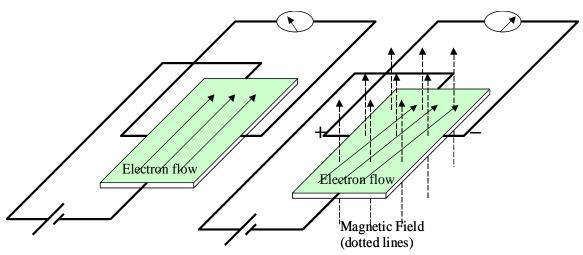
In metals and semiconductors, the effect is quite subtle, but there are materials in which the effect is quite pronounced. There are Hall effect integrated circuits that include sensitive amplifiers and trigger circuits. These are used in electromechanical apparatuses such as DVD players to replace magnetic reed switches. More exotic materials (like "unobtanium") are employed in Hall effect devices have been used in Tektronix clampon DC current probes.
