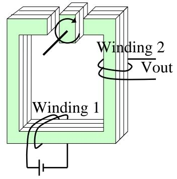
If the iron is not magnetized and there is no current flowing in the coils, nothing remarkable happens. However, if there is a DC magnetic field caused by the battery and winding 1, the magnetic flux in the iron core expands and contracts as the gap is opened
