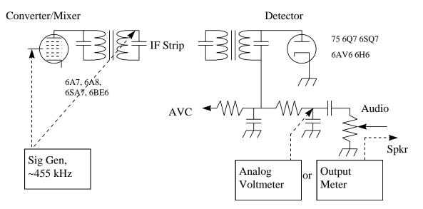
The signal generator amplitude should be advanced until sufficient signal is seen on the meter, and the IF transformers adjusted for peak response. As before, the last IF transformer is done first, and the procedure is repeated on subsequently earlier stages. The signal should be kept just high enough to get a reliable indication on the meter, no higher. Note that the two adjustments in a transformer tend to interact, so it will be necessary to re-peak the adjustments.
