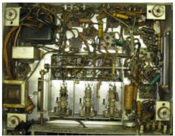
replacement parts were nicely soldered and anchored down were necessary.
