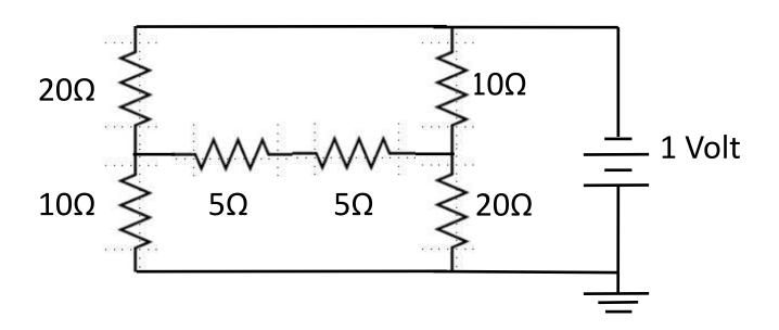
From symmetry, we can determine that the middle node is half way, therefore at 0.5V
