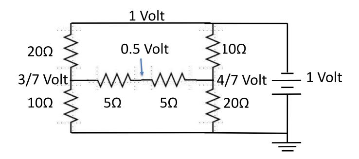
We can calculate the total current now, looking at the two bottom resistors.
