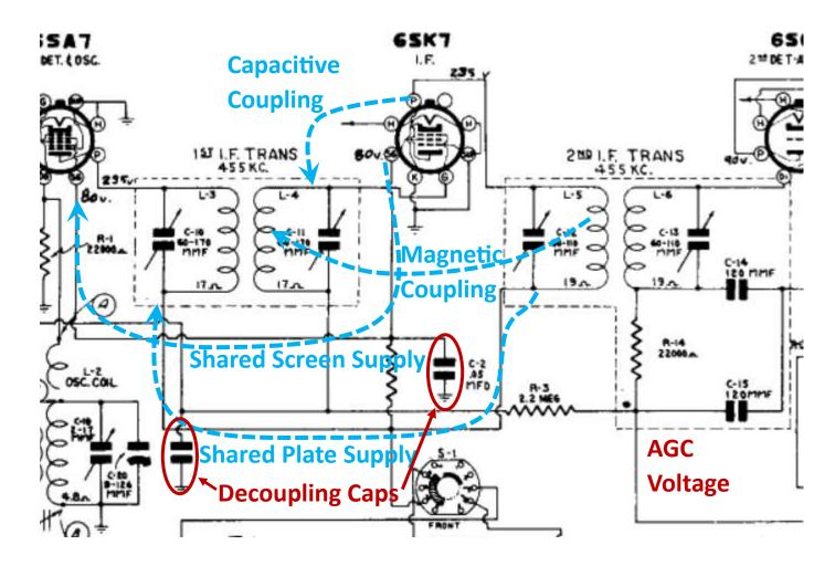
Motorboating (named by the sound it makes) can be caused by an AF oscillation on top of an RF oscillation. An RF oscillation can be so strong that it builds up a DC grid bias voltage that is large enough to turn off the oscillating tube. This stops the oscillation until the DC bias voltage decays, and allows the oscillation to start again, and this can repeat at an audio rate, causing a "growl" or "putt-putt" sound.
