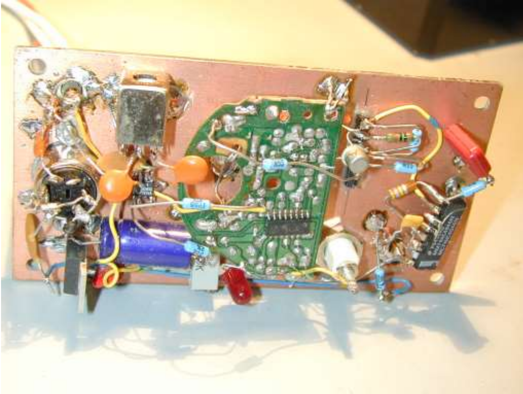
Figure 4: Photograph of the inside of the adaptor. Note that the circuitry surrounding U2 is different than in the schematic.
