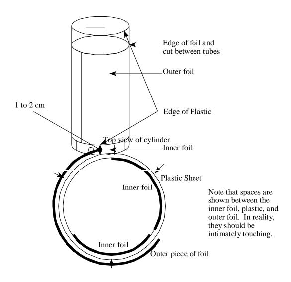
maximiaing the maximum capacitance. This capacitor has a maximum capacitance of about 500pF.
