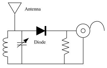
Coil Capacitor Resistor Earphone
