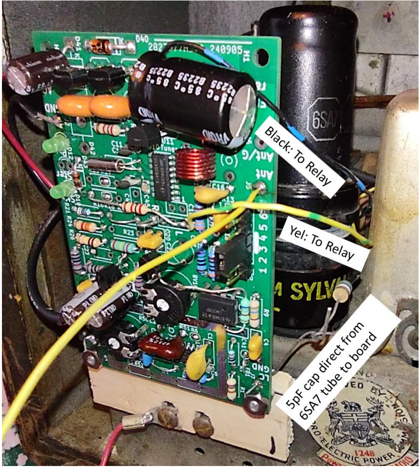
Figure 5 The board on the back of the radio. Held on with the antenna terminals.
