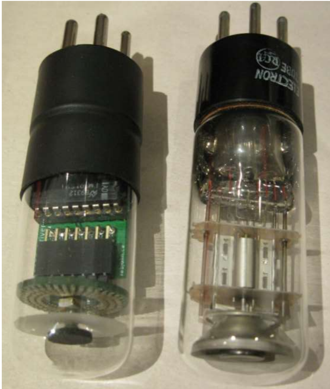
Solid-state tube next to an authentic 6U5.
